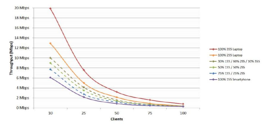
Figure T4-10 Average Per-Device Throughput (AP-225, VHT20, TCP Bidirectional)
